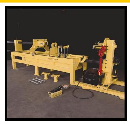
The Tuxco HCS-2520 Hydraulic Cylinder Servicer offers hydraulic cylinder repair facilities a manual model, intended for lower volumes of cylinder repair work. This model is an excellent, low-cost hydraulic cylinder servicer that would prove to be a productive addition to any hydraulic repair facility.
