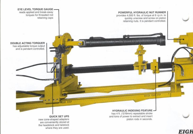
If you frequently repair big, hard to handle and highly torqued cylinders, Tuxco's HCS-60 was designed for you. And while it's built to do the big and tough ones, it is versatile and easy to use on the full spectrum of hydraulic cylinders that a busy shop encounters. No other service bench provides as many hydraulically assisted functions.
