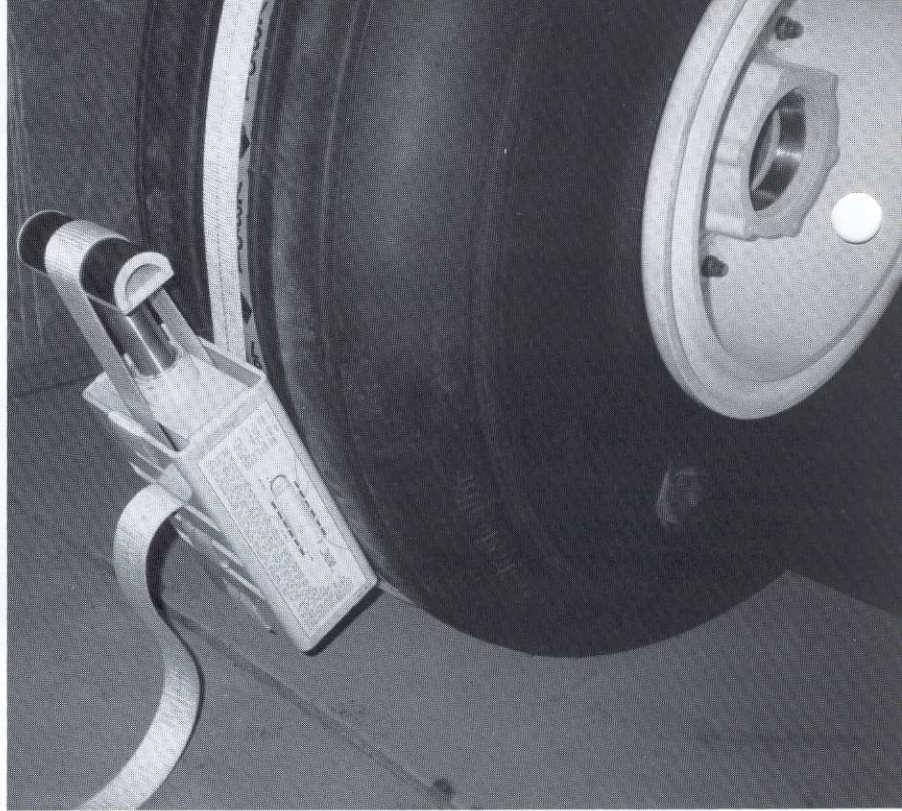
TC-90 shown seating beads of 20.00-20 26 bias ply C-130 AIRCRAFT TIRE.
